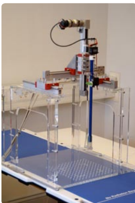
Figure 2. Automatic 3D-moving device for testing random positions.
